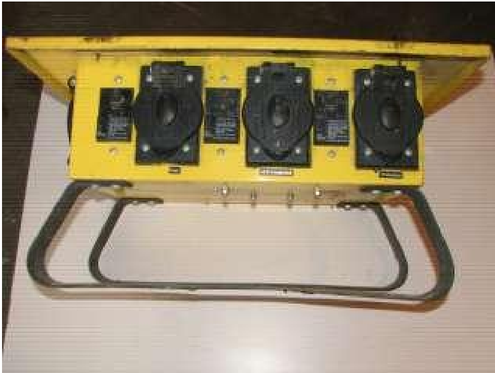
The GFCI appears to the left of the receptacle in this photo.
